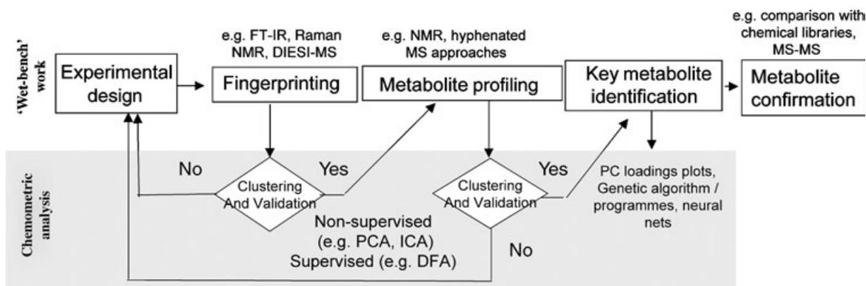
**Figure 10.** A schematic representation of steps undertaken in metabolomic-based analyses to validate the experimental set-up, and to select profiling and chemometric analysis methods in order to confirm metabolite identification.
