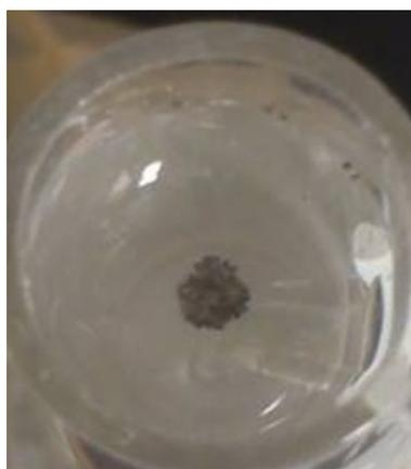
Figure S1: Photograph looking down on the liquid/liquid electrochemical cell following loss of the SERS signal, showing the presence of a silver nanoparticle raft formed, on prolonged potential cycling, at the liquid/air interface
