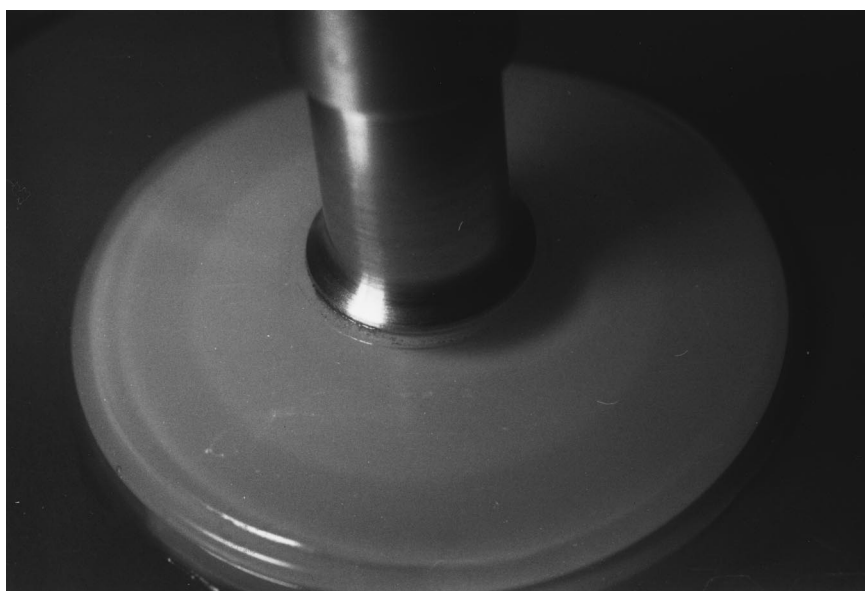
FIG. 3. Photograph of the torsional flow geometry showing the sample has divided into two distinct regions beneath the transparent upper plate. Note that the optical effects at the very edge of the plate are due to a bevel on the plate.
