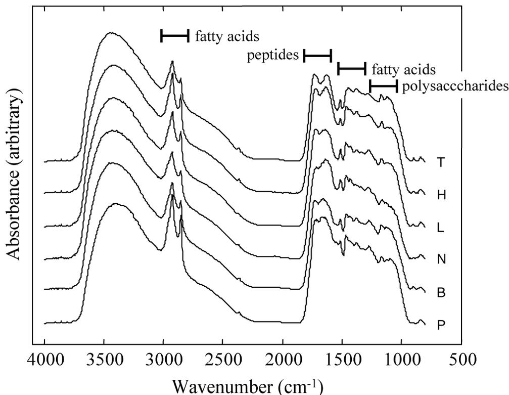
**Fig. 1.** Typical FTIR spectra from the peat samples from the six different locations, encoded T, H, L, N, B and P (see Table I for details). These spectra are offset so that any differences can be more readily observed.
