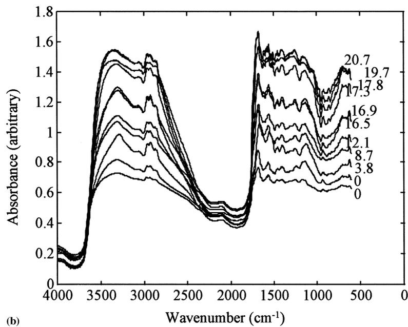
Fig. 2. Diffuse reflectance-absorbance FT-IR spectra (unmanipulated) of (a)  $\alpha 2$  IFN (triplicates) and (b) cell pastes (average of triplicates) with different concentrations of  $\alpha 2$  IFN.
