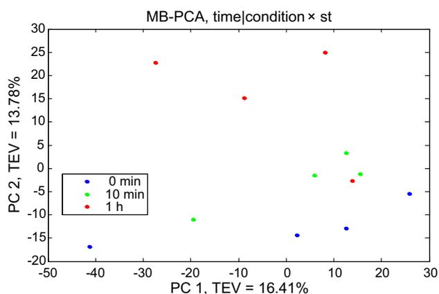
**Fig. 4** MB-PCA scores plot of GC-MS data showing the effect of different time points on *P. putida* strains. Colours represent different time points. 0 min is blue which refers to the point immediately before toluene addition, 10 min in green and 1 h in red refer to the points after 10 min and 60 min of the addition of 0.1 % (v/v) toluene
