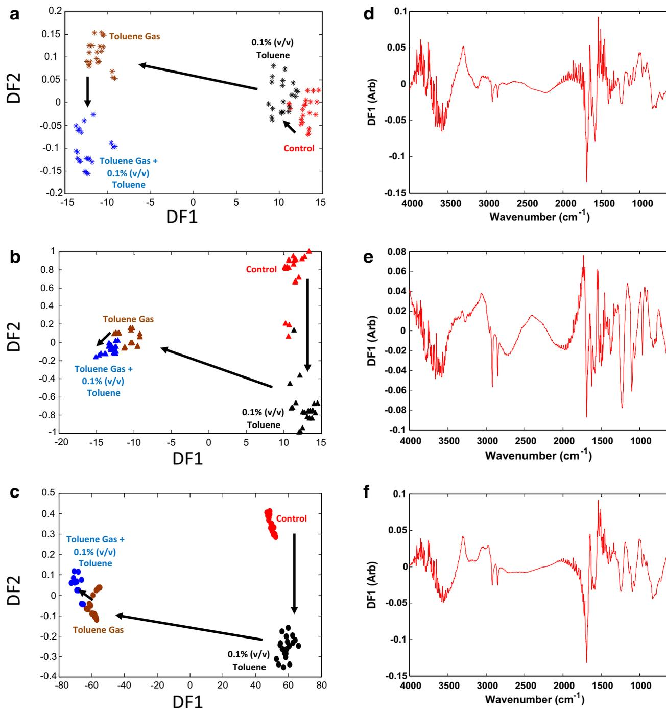
**Fig. 2** PC-DFA scores plots of FT-IR data for three different strains of *P. putida* strains upon toluene stress. Symbols show different strains. **a** *P. putida* DOT-T1E (stars) and the first 10 PCs with a total explained variance (TEV) of 99.94 % were used for the DFA, **b** *P. putida* DOT-T1E-PS28 (triangles) and PCs 1–10 with TEV of 99.93 % were used for the DFA, **c** *P. putida* DOT-T1E-18 (circles) and first 10 PCs with TEV of 99.90 % were used for the DFA.
