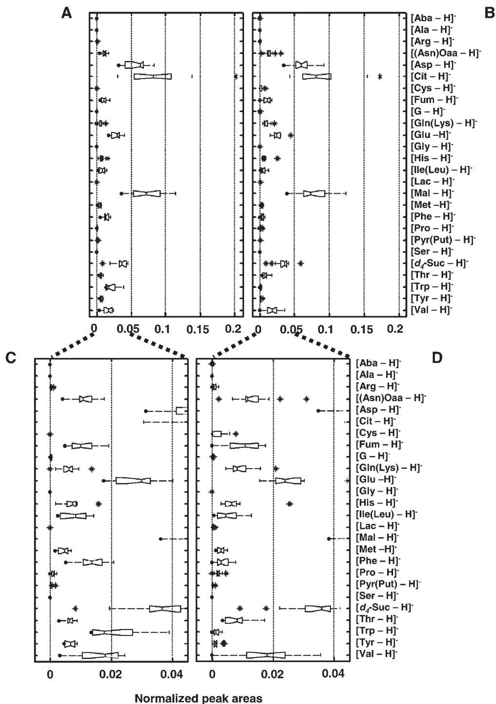
**Figure 4.** Comparison of the median analyte responses on native (A, C) and oxidized (B, D) porous silicon in the negative-ion mode. The response (from 15 replicate measurements) for the analytes in the mixture (cocktail A) is shown as a box-whisker plot. The low response signals can be visualized better in C and D, which contain the same information as in A and B, respectively, but zoomed in for ease of visualization.
