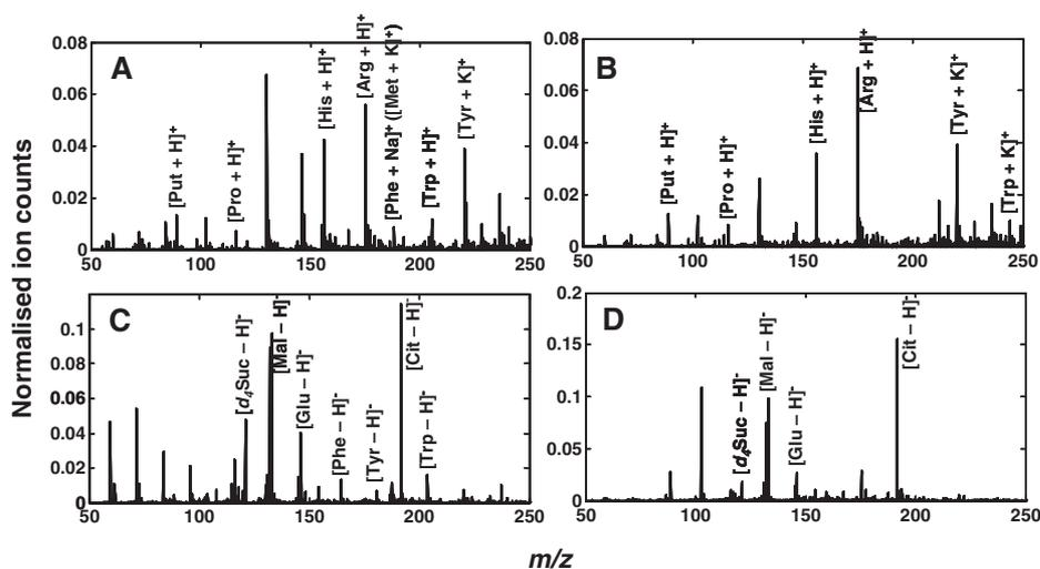
**Figure 1.** Typical laser desorption/ionization mass spectra of the 30-compound cocktail in the positive (A, B) and negative (C, D) ion modes, from native (A, C) and oxidized (B, D) porous silicon surfaces. Peaks corresponding to representative analytes in their protonated, deprotonated or sodium/potassium adduct forms are labeled.
